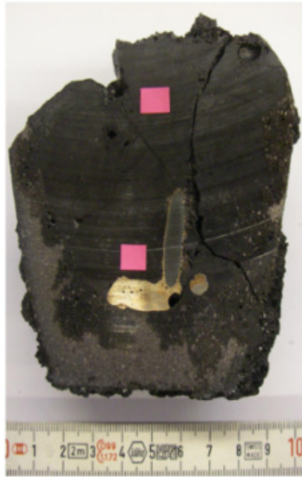
Figure 7: Cross-section of the crucible after the trial with sampled areas marked by the filled rectangles
