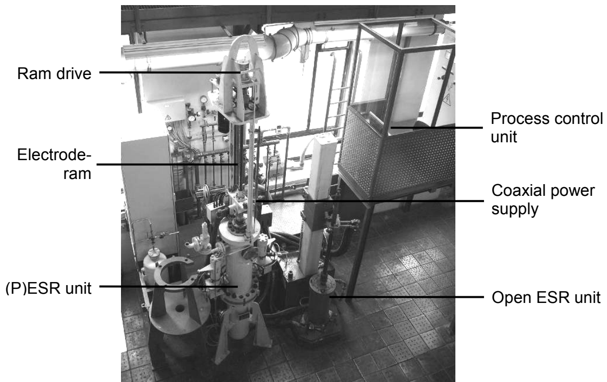
Figure 4: (P)ESR unit at IME Process Metallurgy and Metal Recycling
