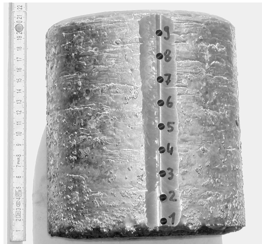
Figure 5: Position of the metal samples in the final ingot
