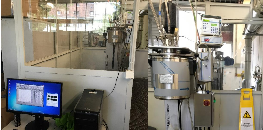
Figure 3: 1 L autoclave with data collection (left) and 10 L autoclave (right)
