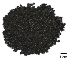
Figure 1: Synthetic fayalitic slag, granulated
