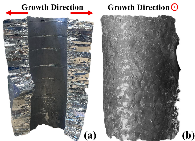
Fig. 10. Surface morphology of crystallised product (a) cross-section (b) solid-liquid interface.
