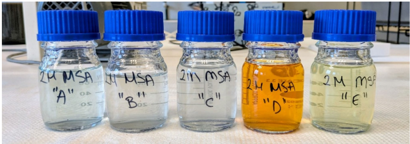
Fig. 6 Leach solutions of different ash samples after 4 h leaching under central leaching conditions (2 M MSA, 40 °C, 1/20 solid-to-liquid ratio). From left to right solutions are in the order of Ash A, Ash B, Ash C, Ash D, and Ash E
